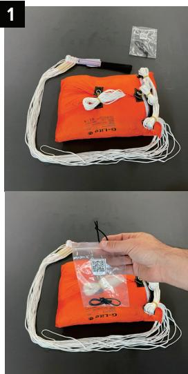
**EN** Prepare the rescue over a clean, dust-free surface, and make sure the lines are not tangled. Take the new elastic textile cords out of the plastic bag.
