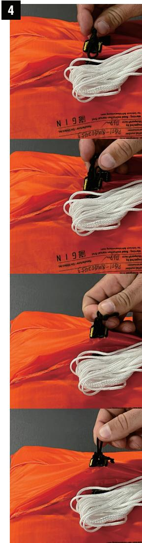
Remove the lark's head knot of the rubber band and also remove the rubber band from the webbing loop.
